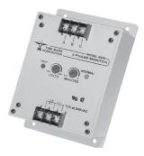
The 265 has two adjustments; one for low voltage, the other for the restart delay. Since the 265 has no trip delay, locations with a poor voltage regulation and/or large inductive loads, will have to have their trip point lowered, to keep from having nuisance trips. The user adjustable restart delay allows up to five minutes for compressor head pressure to bleed off, in the event of short-term power failures. Use of multiple 265's can allow staged restarts if restart times are set differently.
